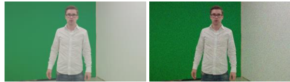
Figure 9: brightness change (left) and salt-and-pepper noise (right)
